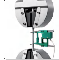
high precision axial extensometer (optional) (a variety of scales can be selected to fully meet the requirements of variety of materials, the accuracy meets class 0.5)
